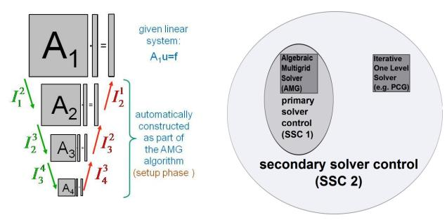
Figure 1: Algebraic multigrid hierarchy (left) and SAMG solver control mechanism
