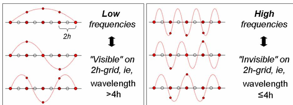
Figure 7: Separation of Fourier components into low (smooth) and high (non-smooth) frequencies, relative to a coarser grid of mesh size  $2h$  (red dots).
