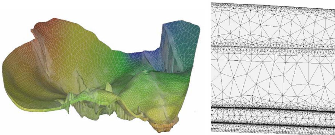
Figure 19: (left) Large-scale 3D basin flow model with unstructured mesh. The pentahedral prismatic mesh necessarily incorporates a number of faulty zones which leads to a vertical distortion of the prisms along these locations. (right) A complex cross-sectional 2D problem. The triangular mesh is fully unstructured and locally refined in a layered geometry. The problem models an aquifer-aquitard system with heterogeneous distribution of conductivity and storativity. (Courtesy of Wasy GmbH)
