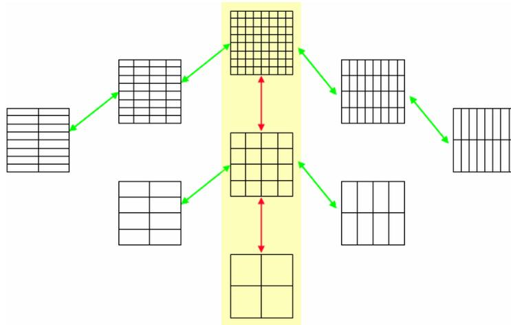
Figure 16: Outline of multiple semi-coarsening strategy for anisotropic problems in connection with plain GS smoothing
