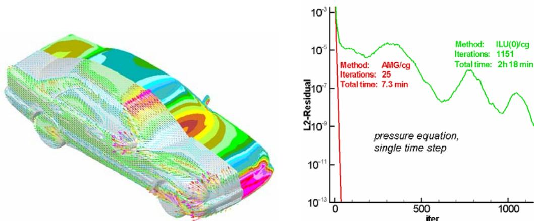
Figure 28: (left) Mercedes-Benz E-Class model. (right) Comparison of convergence histories between SAMG and a standard one-level solver. (Courtesy of Daimler-Benz and Computational Dynamics)
