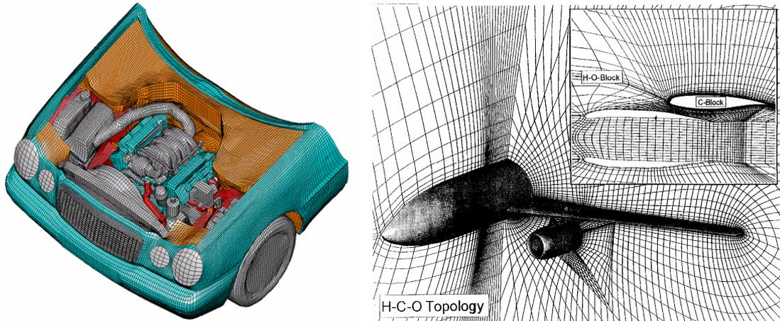
Figure 1: Grids for computing the underhood flow (left; courtesy of Computational Dynamics and Daimler-Benz) and the flow around an aircraft (right).
