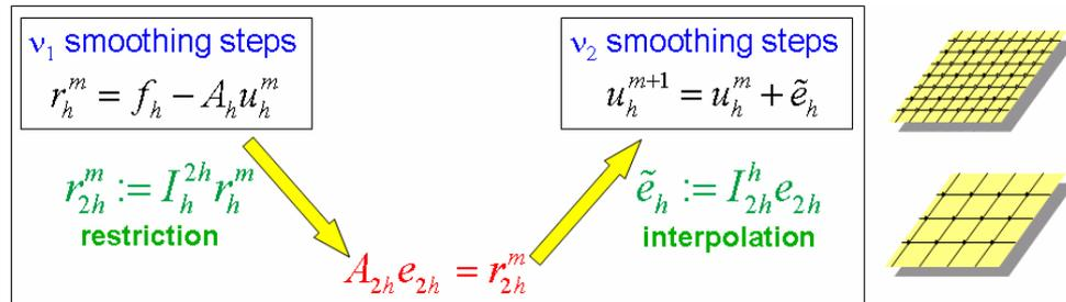
Figure 9: Mathematical description of a two-grid method
