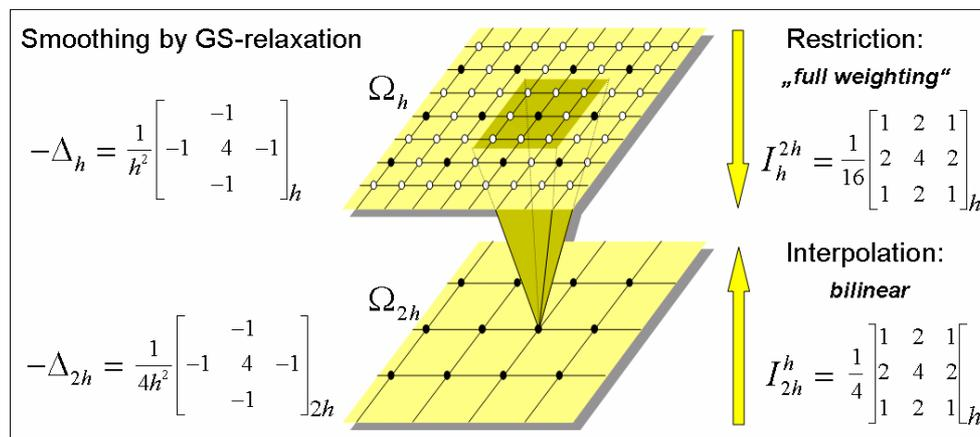
Figure 10: Reasonable components defining a two-grid method for solving Poisson equation. The special fine-to-coarse averaging is usually called “full weighting”; the coarse-to-fine mapping is just bi-linear interpolation.
