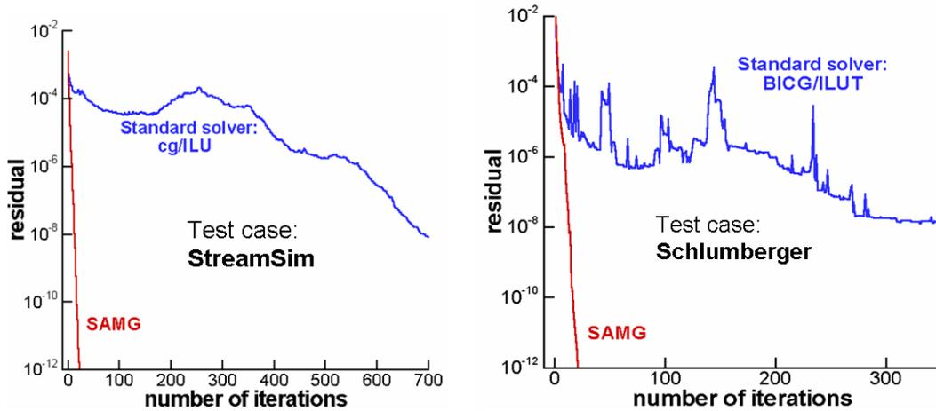
Figure 31: Comparison of SAMG’s convergence history with that of a standard one-level method in solving the pressure equation in the streamline approach. The figures correspond to a symmetric (left) and non-symmetric (right) test case.
