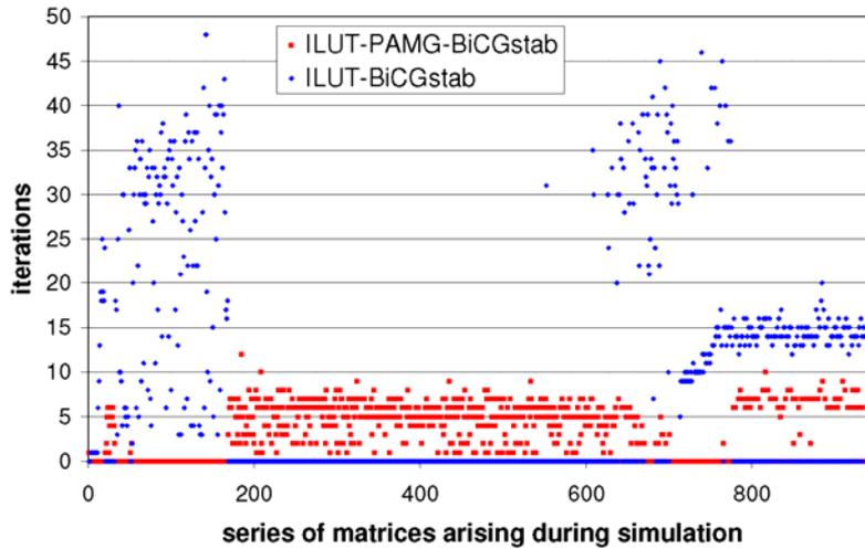
Figure 35: Solver switching and number of iterations for Case C1. Both, one-level (blue dots) and multi-level (red dots) methods are chosen by  $\alpha$ -SAMG.
