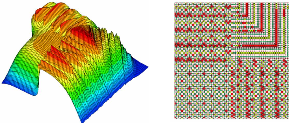
Figure 27: (left) “Smooth” error in case of Problem (19). (right) The finest and three consecutive levels created by the standard SAMG coarsening algorithm.
