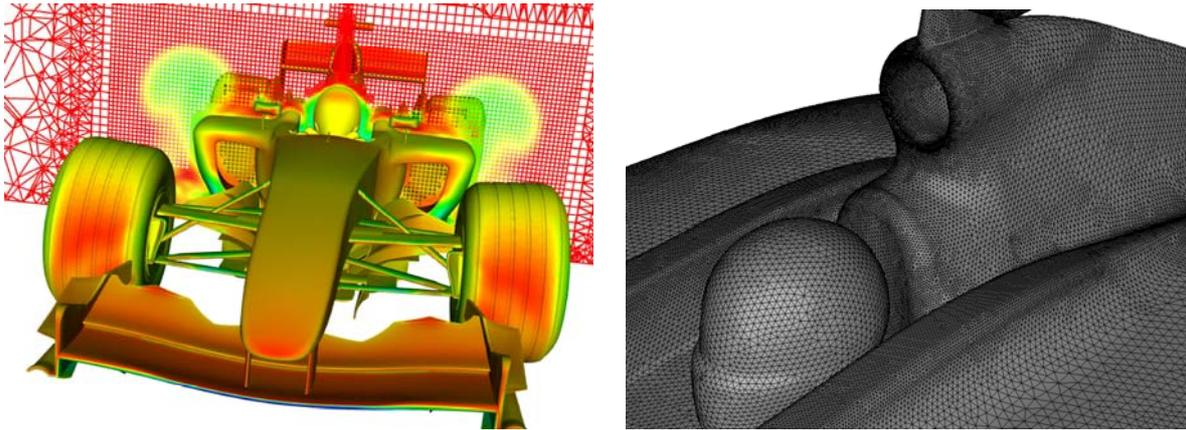
Figure 2: (left) Cross section of a highly complex mesh for the simulation of the exterior flow around a racing car. (right) Corresponding surface mesh near the driver. (Courtesy of Fluent and Sauber-Petronas)
