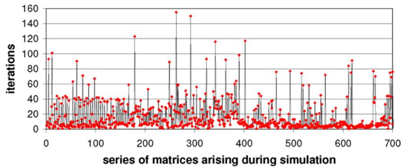
Figure 37: Number of SAMG iterations for Case C2. Only real multi-level methods are chosen by  $\alpha$ -SAMG, one-level variants are not competitive.
