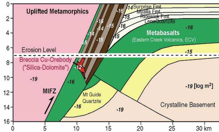
Figure 14: Drastic changes in permeabilities causing discontinuous coefficients
