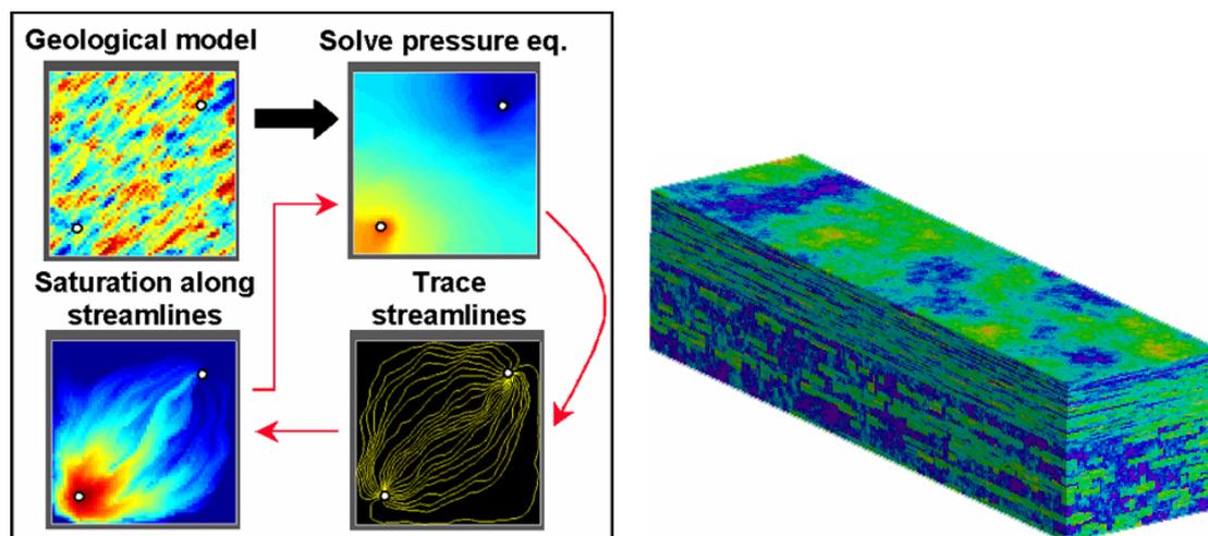
Figure 30: (left) Schematic view of the streamline approach. (right) SPE 10 upscaling benchmark model, 1.12 million cells.
