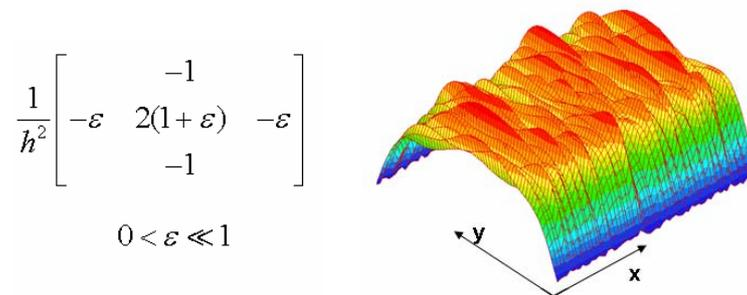
Figure 12: Error smoothing by GS relaxation applied to the anisotropic Poisson equation (7). Starting from a random first guess, the error gets quickly smooth only in the *y-direction* (i.e. in the direction of “strong connections”).
