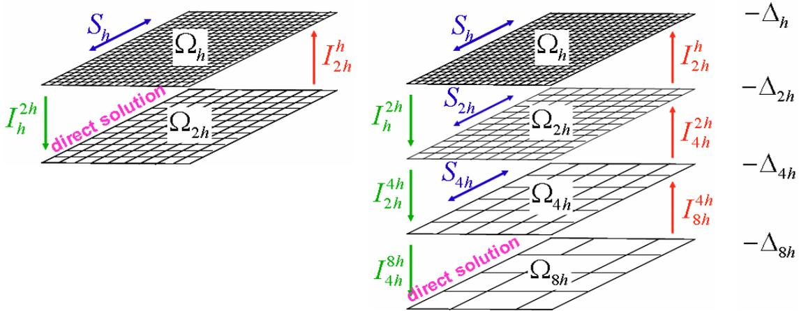
Figure 11: (left) Schematic view of two-grid method. (right) Recursive extension of the two-grid method to a multigrid method.
