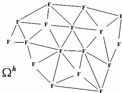
Figure 18: Graph representation of a matrix: The nodes of the graph stand for the variables; edges for non-vanishing couplings between variables. In analogy to the finest grid in the context of GMG, we denote this graph by  $\Omega^h$ . “F” stands for fine level nodes.
