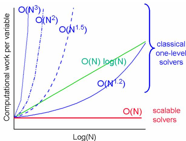
Figure 3: Computational work (scaled by the number of variables) for different types of solvers.
