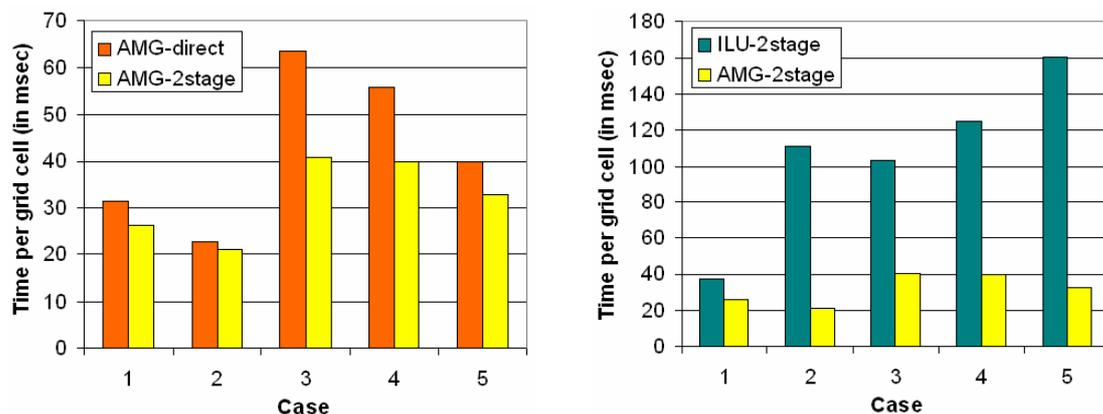
Figure 32: Oil-water simulations: (left) Comparing AMG solver strategies. (right) Comparing AMG with multilevel ILU [3] for solving the pressure equation in a two-stage preconditioning approach.
