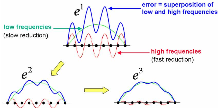
Figure 8: Illustration of how relaxation acts on some error which is the superposition of a low and a high frequency component.
