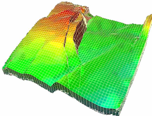
Figure 34: Type of grid used by the SURE simulator (Voronoi grid; courtesy SMT Alps)
