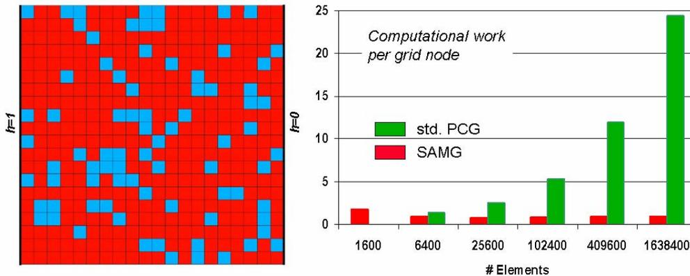
Figure 29: Durlafsky problem: (left) Conductivity pattern (red= $1\text{m/s}$ ; blue= $10^{-6}\text{ m/s}$ ), basic  $20\times 20$  mesh. (right) Performance of SAMG compared to that of a standard one-level solver for increasing mesh size.
