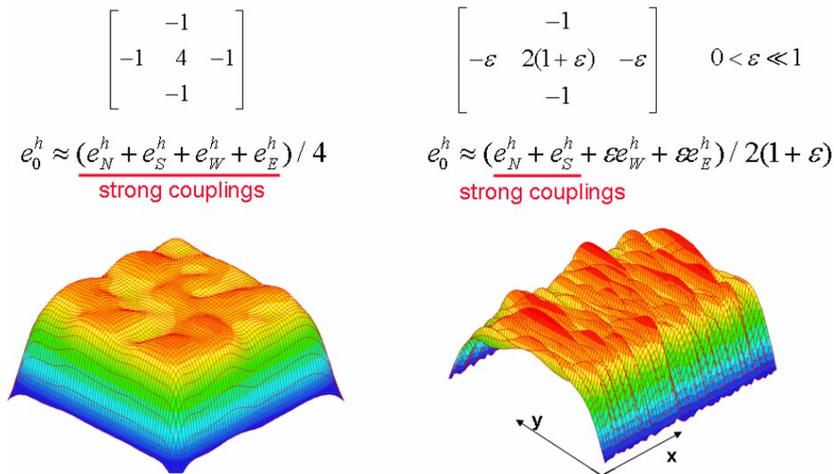
Figure 20: Visualization of algebraic smoothness for isotropic and anisotropic problems
