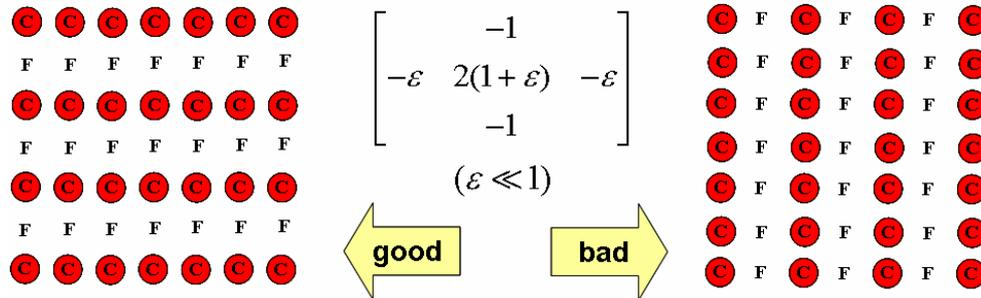
Figure 21: Meaning of ‘‘coarsening in the direction of strong couplings’’ in case of the anisotropic model operator.
