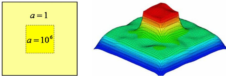
Figure 13: (left) Definition of discontinuous coefficient  $a$  in (9). (right) “Smooth” error obtained after a few sweeps of GS relaxation starting with a random guess.
