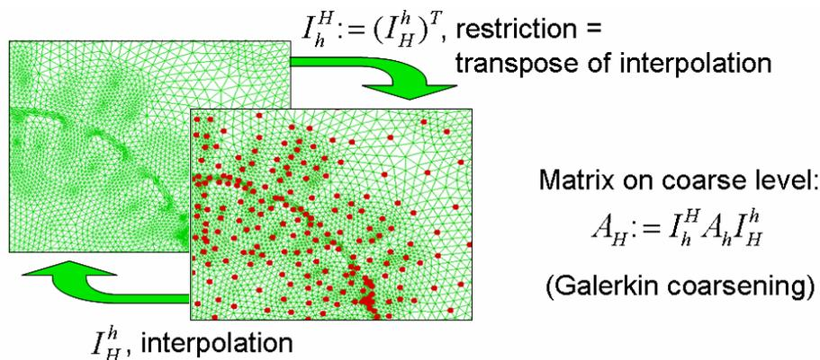
Figure 24: The ingredients of a two-level method
