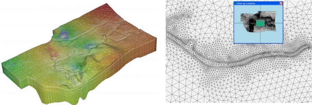
*Figure 4: Large-scale 3D flow model with unstructured mesh. This can be considered as a typical transient finite-element groundwater model used in practical water resources simulation. (Courtesy of Wasy GmbH)*
