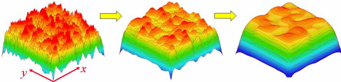
Figure 6: The shape of the error for the very first relaxation sweeps, starting from a random first guess.
